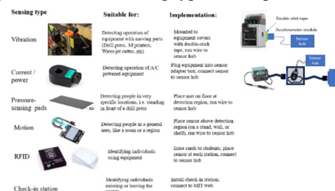
Figure 1: Summary of the six sensing types explored for instrumentation
