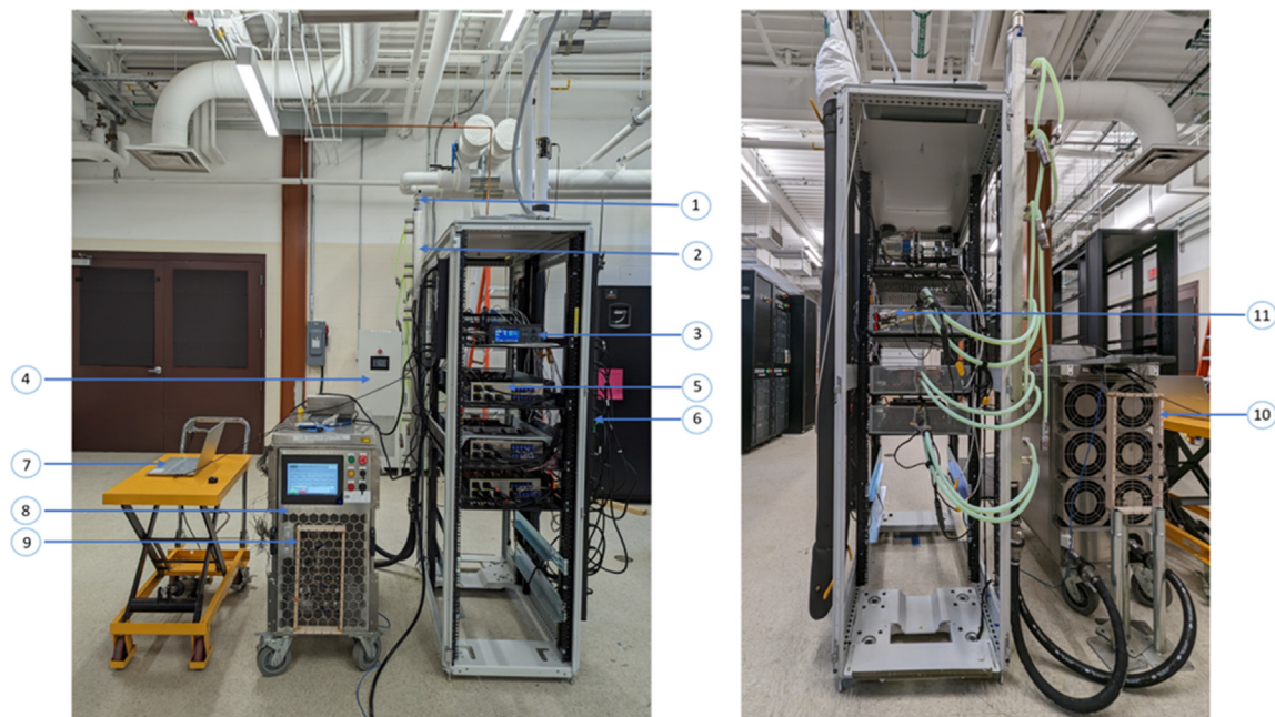
Fig. 1 The experimental setup for the liquid-to-air CDUs. Components: (1) rack manifold's air vent, (2) rack manifold, (3) data acquisition system, (4) power supply, (5) TTVs, (6) power distribution unit, (7) laptop, (8) liquid-to-air CDU, (9) thermocouple mesh for air side measurements (inlet), (10) thermocouple mesh for air side measurements (outlet), and (11) CLs inlet and outlet instrumentation.
