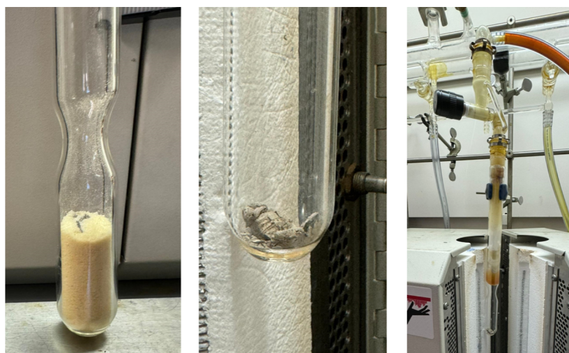
Figure 2. Images collected from the small-scale synthesis of yttrium triiodide. Left: the mixture of yttrium metal pieces and ammonium iodide before heating under argon. Center: large pieces of yttrium triiodide after the decomposition of (\text{NH}_4)_3\text{YI}_6 under reduced pressure. Right: Excess ammonium iodide collected in the upper part of the apparatus and completely separated from the yttrium triiodide.
