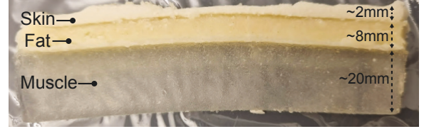
Fig. 5. Cross-section view of the fabricated multi-layer phantom.
