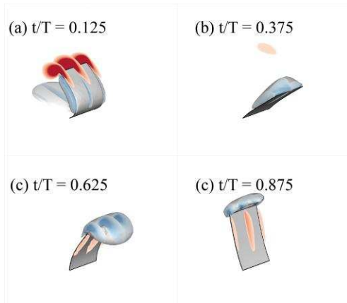
Figure 9. Isosurface of Q criterion and chordwise vorticity at t/T = 0.125, 0.375, 0.625, \text{ and } 0.875 .
