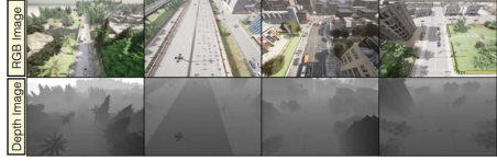
Fig. 5. SKYSCENES RGB Images and corresponding depth images generated using depth sensor for h = 35 , \theta = 45^\circ , and ClearNoon setting across four different town layouts.
