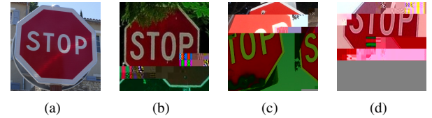
Fig. 2. Examples of images distorted by different packet loss and buffer overflow during their network communication: (a) – original stop sign image; (b) – stop sign image transmitted with buffer 128B and 5% packet loss; (c) – stop sign image transmitted with buffer 256B and 5% packet loss; (d) – stop sign image transmitted with buffer 512B and 20% packet loss
