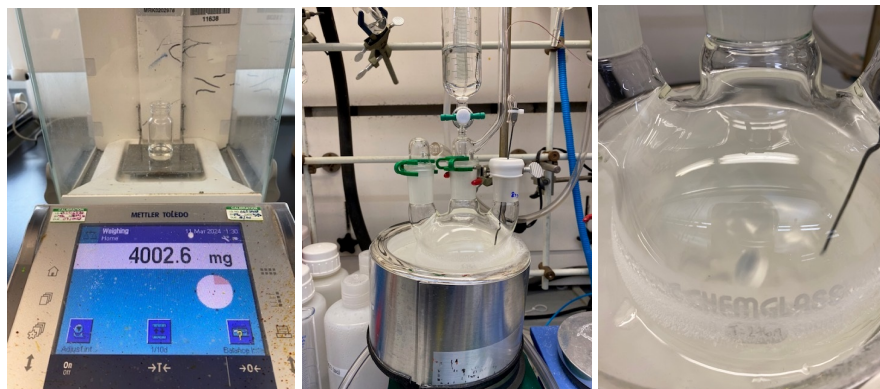
Figure 1. (A) N -Boc-D-Proline methyl ester weighed in 20 ml vial; (B) Reaction assembly; (C) Reaction mixture before DIBAL-H addition (photos provided by checkers)
