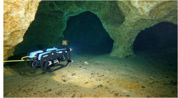
Fig. 1: A BlueROV2 is operating inside an underwater cave system by following its caveline in Orange Grove, FL.
