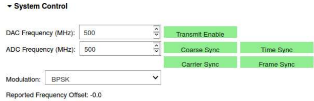
Fig. 5. The radio control interface: manages transmission start/stop, phase timing, and frame synchronization, ensuring precise and synchronized signal handling.
