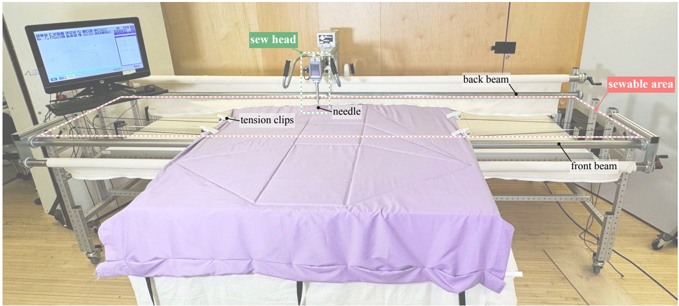
Figure 3: A computer-controlled long-arm sewing machine for quilting.
