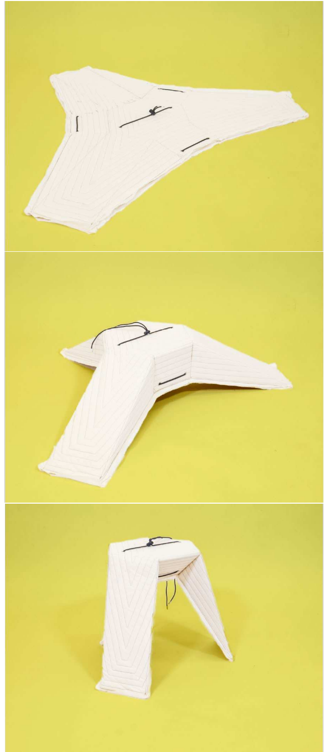
Figure 2: This side table folds from flat to its 17"-tall ( \approx 43 cm) final shape when a cord laced through grommets is pulled. (Materials: quilted muslin-batting-muslin top fabric, 3/16" plywood inserts, muslin backing fabric.)
