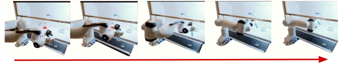
Fig. 9: The robot transporting a graduated cylinder into the fume hood while avoiding spills and collisions
