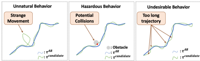
Fig. 3: Visualized candidate demonstrations may exhibit behaviors that could lead to rejection by the user: (left) unnatural motions due to poor IK solutions, (middle) potentially hazardous motions, (right) misalignment with the user’s preferences.
