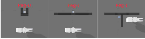
Fig. 4. The peg-in-hole environments. The end-effector is grasping a peg, which the robot navigates to the hole. Environments and figure are from [12].
