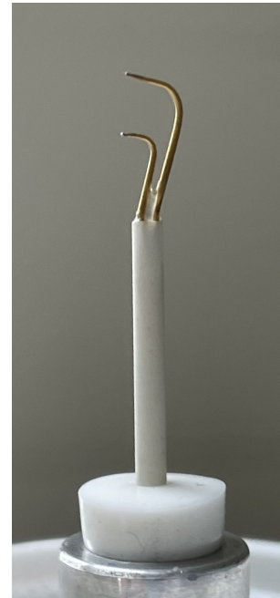
Figure 1. UFT-2B head sensor. Parallel to the mean flow, tungsten wire (2.5 \mu\text{m} thick, 3 mm long) spanned a miniature industry standard wire probe by DANTEC ® .
