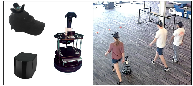
Fig. 1. (left) Our tracking solution includes Vive Trackers 2018 attached to hats, a Vive Controller mounted on a Turtlebot, and Vive Base Stations 2.0. (right) A still from the overhead webcam during an experimental trial.
