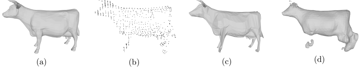
Fig. 13 (a) Original Cow. (b) Point cloud with a 65% reduction. (c) Reconstruction using our method, Algorithm 1. (d) Reconstruction using MeshLab [26].
