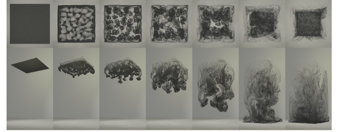
Fig. 13. Two Drop Interaction. At a high Reynolds Number, two drops interact and form a complex pattern.
