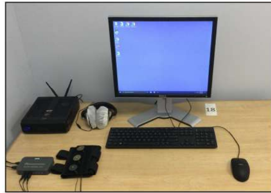
Fig. 2. Experimental setup and hardware used (From top left clockwise: headphones, monitor, keyboard, mouse, armband with tactors, C-2 tactor box).
