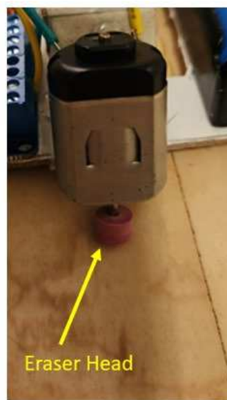
Figure 2-13: Close Up of Eraser Head on Axle of Motor 1
