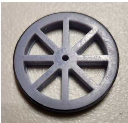
Figure 2-15: 3D Printed Wheel – Left diagram shows wheel face with 3 cm diameter and the diagram on the right shows the black band on the wheel's rim.
