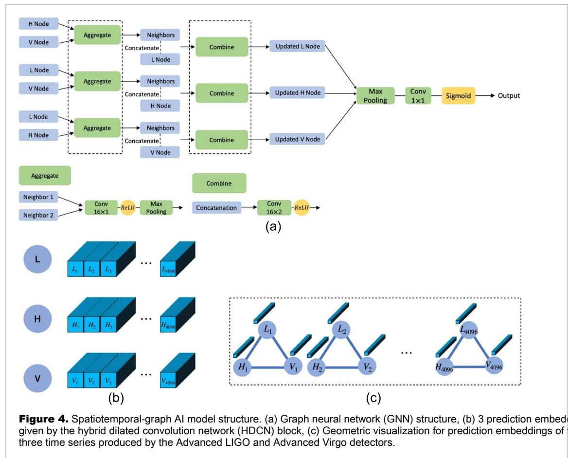
**Figure 4.** Spatiotemporal-graph AI model structure. (a) Graph neural network (GNN) structure, (b) 3 prediction embeddings given by the hybrid dilated convolution network (HDCN) block, (c) Geometric visualization for prediction embeddings of the three time series produced by the Advanced LIGO and Advanced Virgo detectors.
