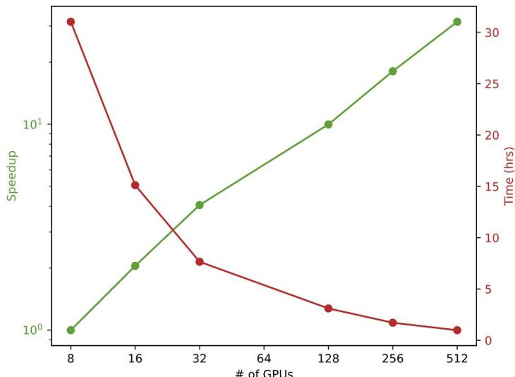
**Figure 5.** Distributed training in the Polaris supercomputer. We developed novel methods to complete the training of spatiotemporal-graph AI models within 1.7 h using 256 A100 NVIDIA GPUs. Our optimization method exhibits strong scaling up to 512 NVIDIA A100 GPUs.
