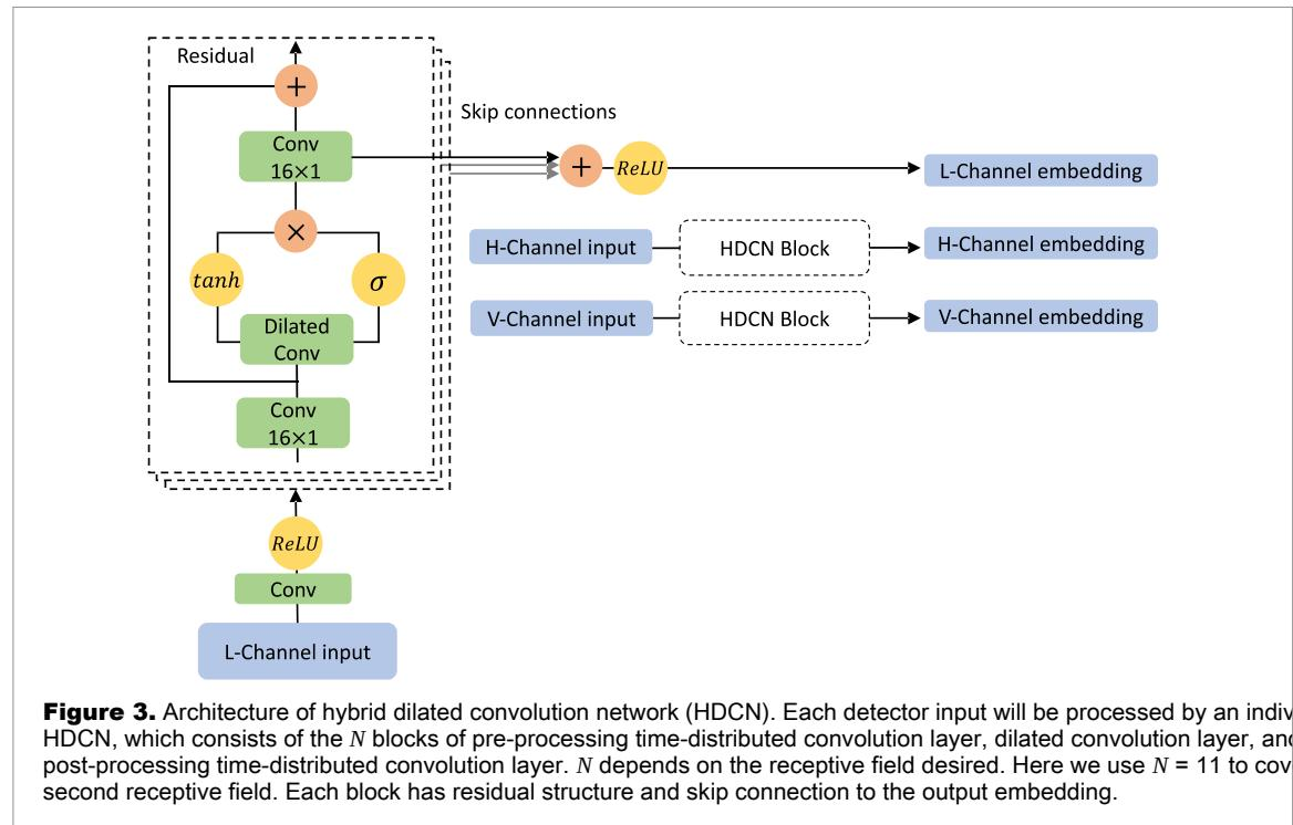
**Figure 3.** Architecture of hybrid dilated convolution network (HDCN). Each detector input will be processed by an individual HDCN, which consists of the  $N$  blocks of pre-processing time-distributed convolution layer, dilated convolution layer, and the post-processing time-distributed convolution layer.  $N$  depends on the receptive field desired. Here we use  $N = 11$  to cover a half second receptive field. Each block has residual structure and skip connection to the output embedding.
