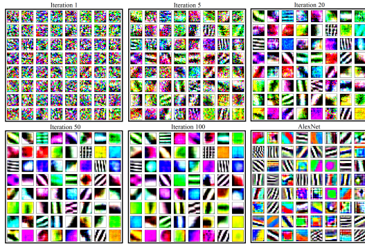
FIGURE 7: Visualizations of the 11 \times 11 weights of the 64 features in the CNN layer of CG-CNN after 1, 5, 20, 50, and 100 EM iterations. Also shown are the weights of the 64 features in the first layer of AlexNet. While even after 20 EM iterations the features are still quite crude, the features at iterations 50 and 100 are sharp and almost identical and resemble AlexNet features.
