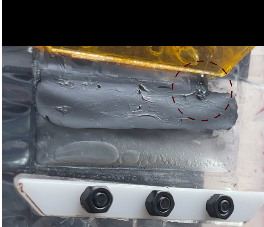
Figure 3.2: Charge accumulation at the boundary of the film and electrode visible on the top right corner of the electrode layer (gray).
