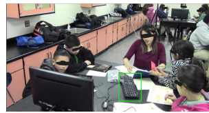
(b) Successful typing region proposal using keyboard tracking when keyboard is fully visible.
