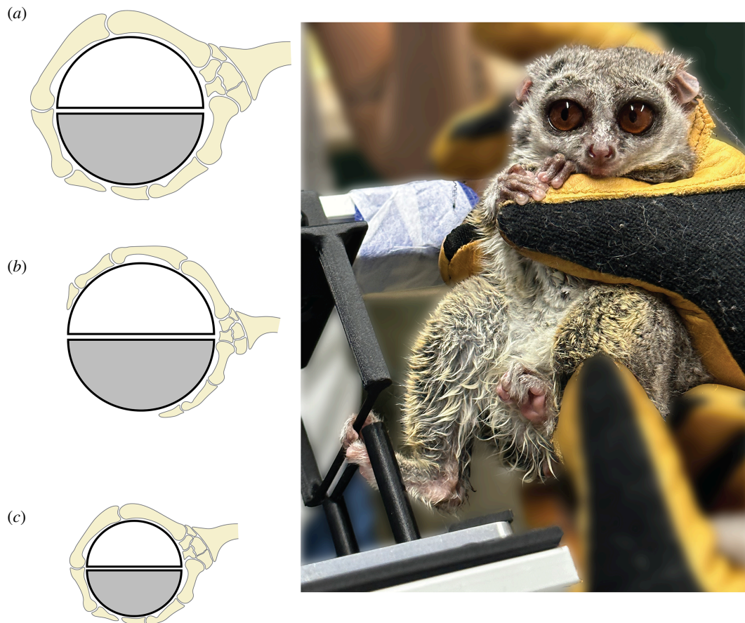
Figure 1. Schematic of the experimental setup and ideal autopodial wrapping posture (a). The substrate that the animals gripped consisted of two carbon fibre-embedded, 3D-printed semi-lunar bisections. The upper portion (white) of the substrate was uninstrumented and provided a solid anchor on which the autopodia could rest. The lower portion (shaded) was affixed to a force plate and recorded an upward force as the animal grasped. See Dickinson et al. [10] and Young et al. [11] for a more detailed representation of the experimental setup. Instead of using the same substrate size across species, which could lead to underwrapping or overwrapping of the digits (b), the substrate size was adjusted for each individual to maintain a physiologically equivalent grasping posture regardless of the individual's size (c). Animals were positioned so that body mass did not rest on the instrumented portion of the force plate, thus ensuring that only grasping forces were recorded.
