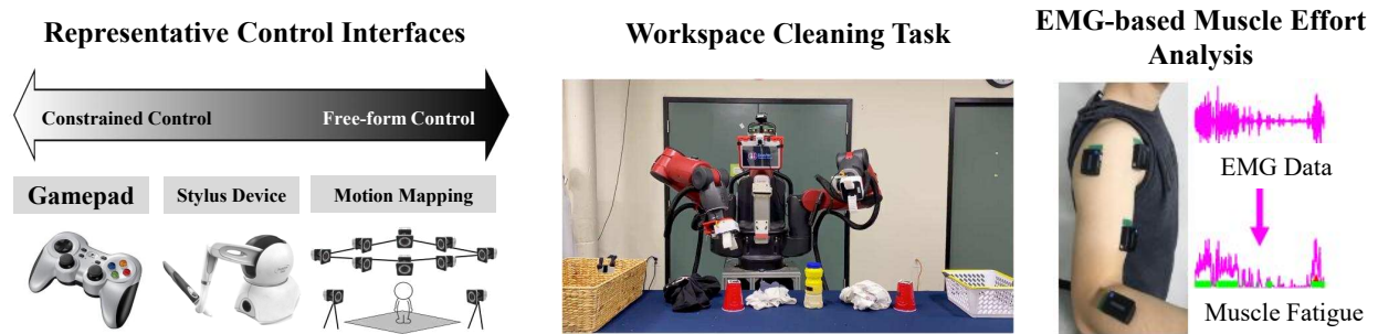
Figure 1.2: (From left-right) Representative control interfaces evaluated in user study across spectrum of constrained to free-form control [2]; Workspace clearing task; Muscle effort analysis using EMG sensors.
