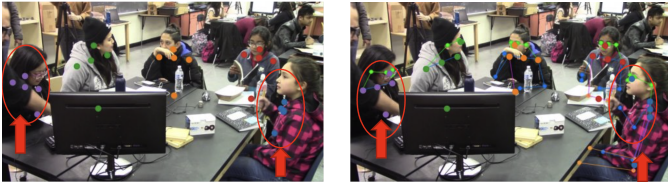
Fig. 4: Robust 3D Pose estimation using YOLO and PoseNet. The left image shows the results for PosNet alone. Right image shows the results when using PoseNet with YOLO.
