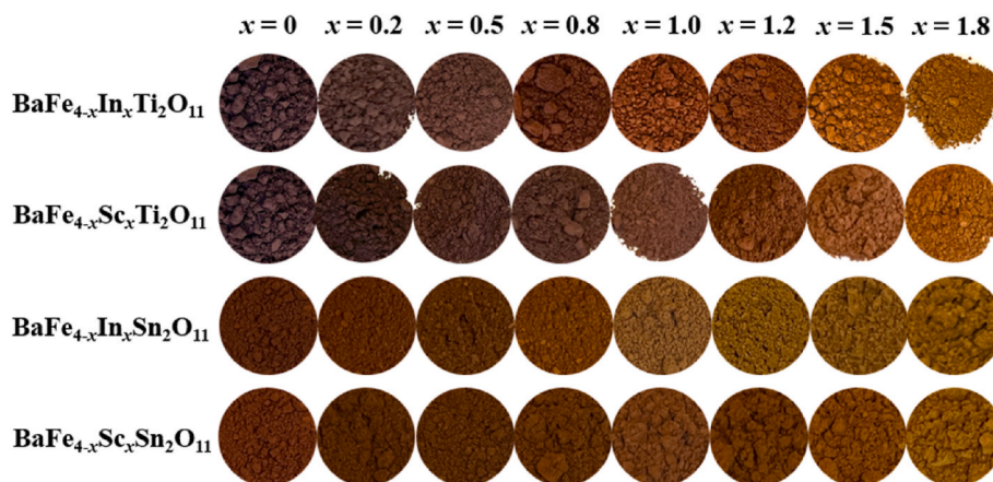
Fig. 9. The corresponding sample colors of the new solid solutions with R -type hexaferrite structure, with the nominal composition \text{BaFe}_{4-x}\text{M}_x\text{M}'_2\text{O}_{11} .
