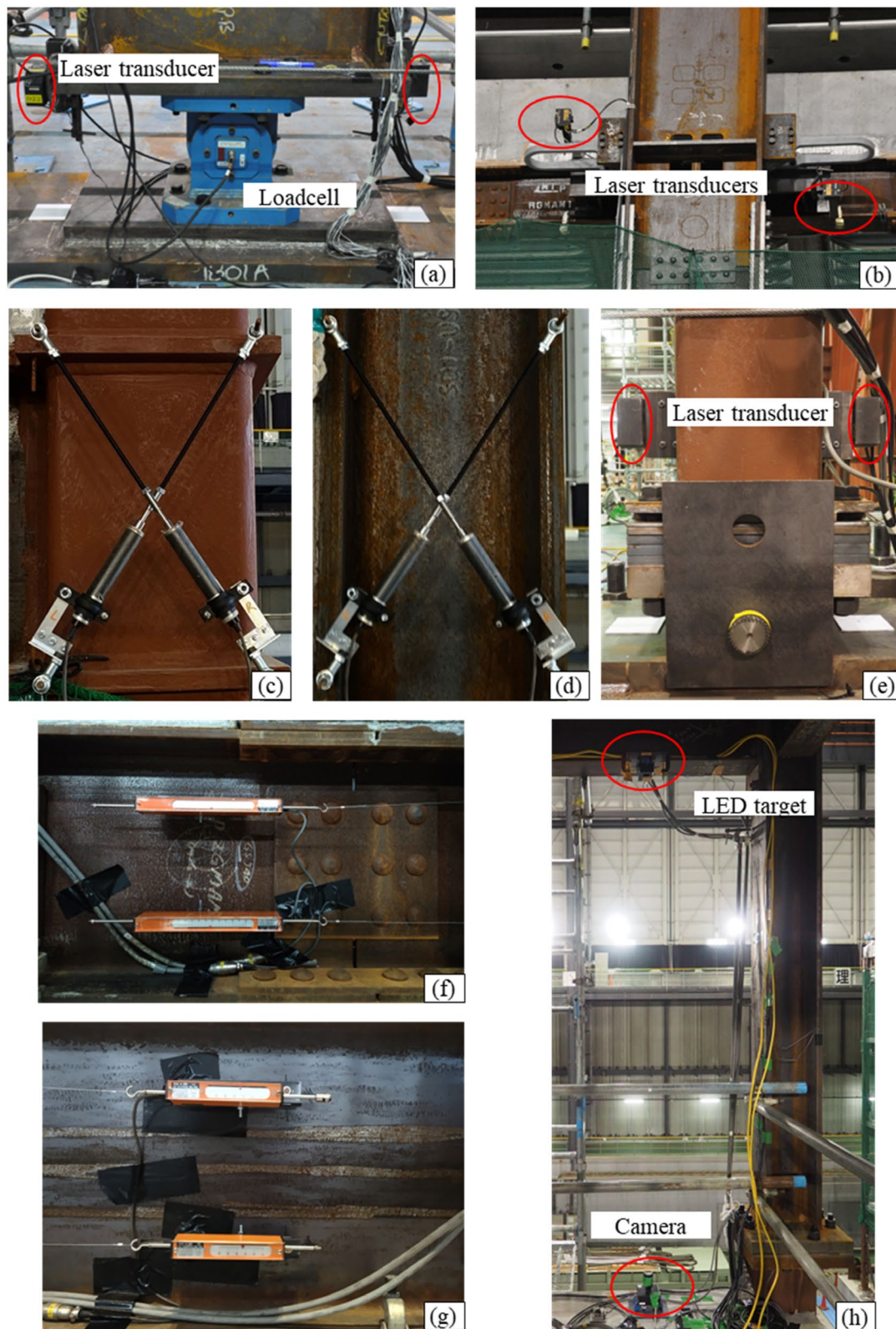
FIGURE 9 | Photos of instrumentation: (a) load cell and rotation at pinned base of Spine; (b) horizontal displacement at MRF-to-Spine connection; (c, d) shear deformation of column panel zone; (e) rotation of column base; (f, g) rotation of beam end; (h) optical system.
