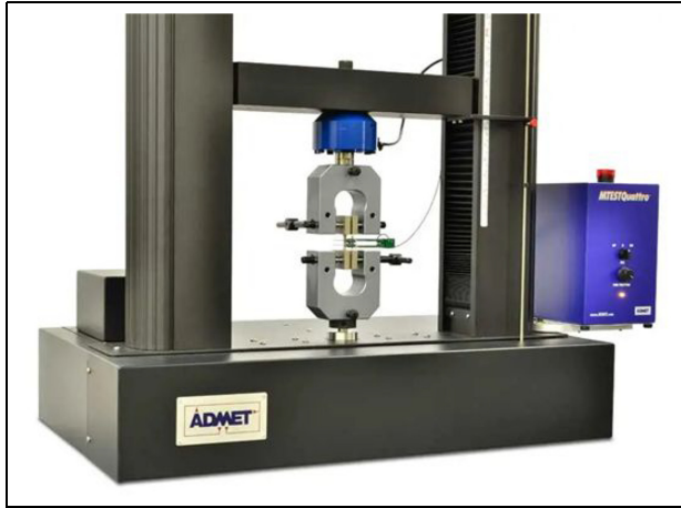
Figure 4. ADMET Expert 2653 tensile and compression testing machine.
