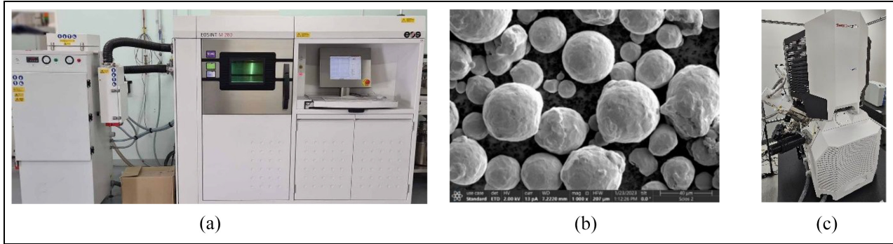
Figure 1. Metal 3D printing system and SEM and image of maraging steel powder: (a) EOSINT M280 machine, (b) SEM imagery of EOS MS1, (c) SCIOS_2 SEM.
