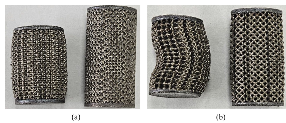
Figure 16. Compression deformation close-up of BCC and FCC topologies: (a) BCC topology, (b) FCC topology.
