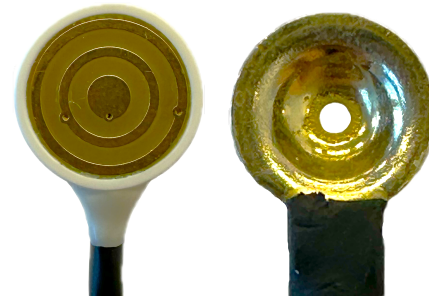
Fig. 1. (Left) tEEG electrode. (Right) Conventional EEG electrode.
