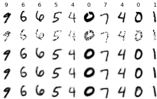
Fig. 11: Random examples from the MNIST test set, random zeroed images and the reconstructions from the denoising models. The first row lists the raw examples. The second row lists the zero noised images. The third row shows denoised images from the DAE. The fourth row shows denoised images from the DSDAE. The fifth row shows the denoised images from the sparse DSDAE.
