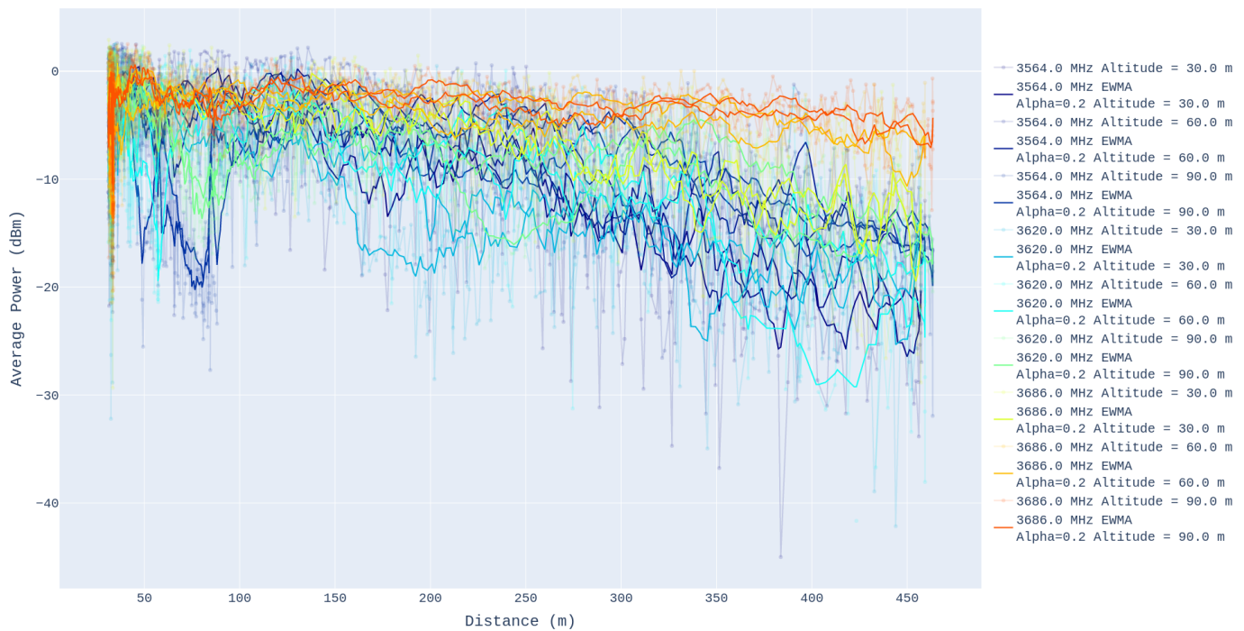
Fig. 7: Received signal power values over distance at different altitudes and frequencies.
