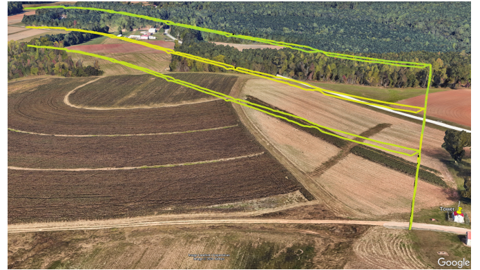
Fig. 5: The three flight paths of the UAV at constant altitudes of 30m, 60m, and 90m above ground level at the starting location.
