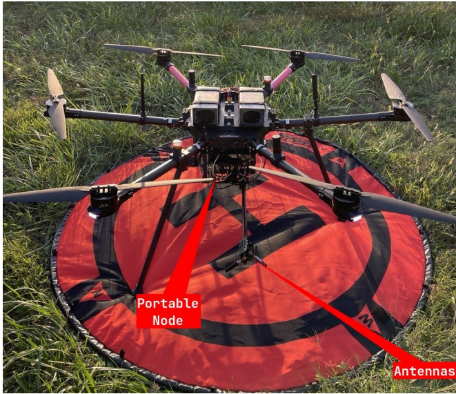
Fig. 3: The UAV and portable node used for the measurements.
