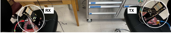
Fig. 7. Beam-sweeping experiment setup with transmitter and receiver software-defined arrays (SDAs) placed at a distance of 4.5 m in an indoor environment. The distance in the image is not to scale.
