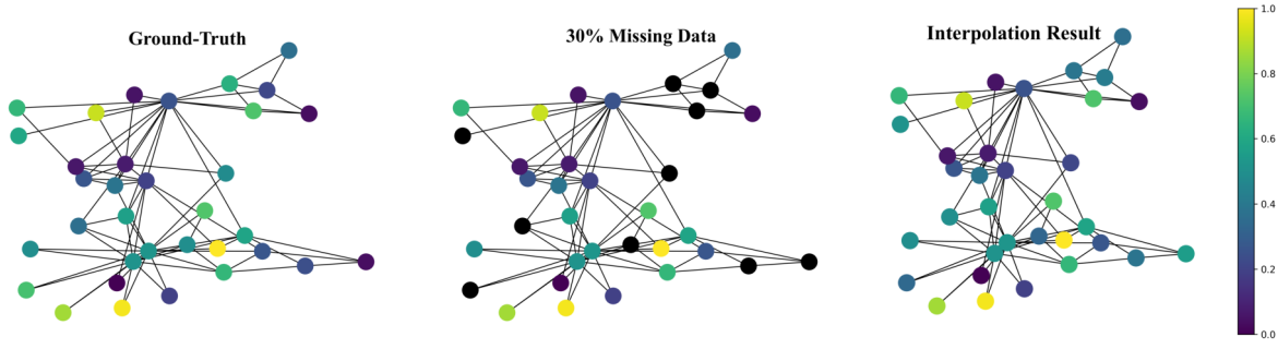
Fig. 3: Heat map on the normalized values of graph signals within the range of [0, 1] . Left: the ground-truth data. Middle: the model input with 30% of the data missing. Right: the interpolation result achieved by our algorithm.
