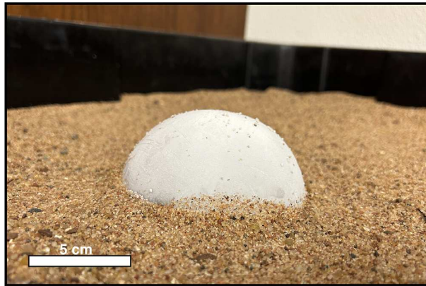
FIGURE 2 Profile image of a 10-cm ice sphere half-buried within a container of well-sorted, coarse sand. The bottom of the ice sphere is positioned at a depth equal to one radius (5 cm) below the sand surface, with approximately half the sphere protruding above the sand surface. [Color figure can be viewed at wileyonlinelibrary.com ]
