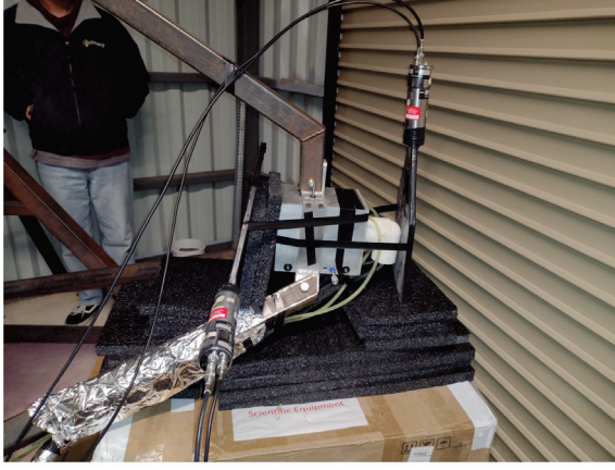
(a) Horizontal muon paddle configuration.
