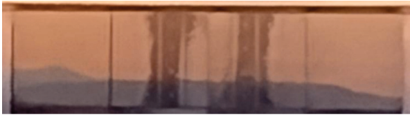
Fig. 18. Image of the first row of SiPM matrices ( 4 \times 16 SiPM camera pixels) taken after sunset. Imaged onto the SiPM camera by the telescope optics is the mountain range in the west at which the Demonstrator points. The ridge is clearly resolved, demonstrating the optical performance of the Demonstrator. The dark vertical lines in the middle are reflection artifacts.
