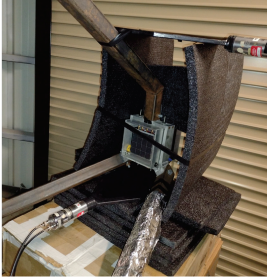
(b) Vertical muon paddle configuration.
