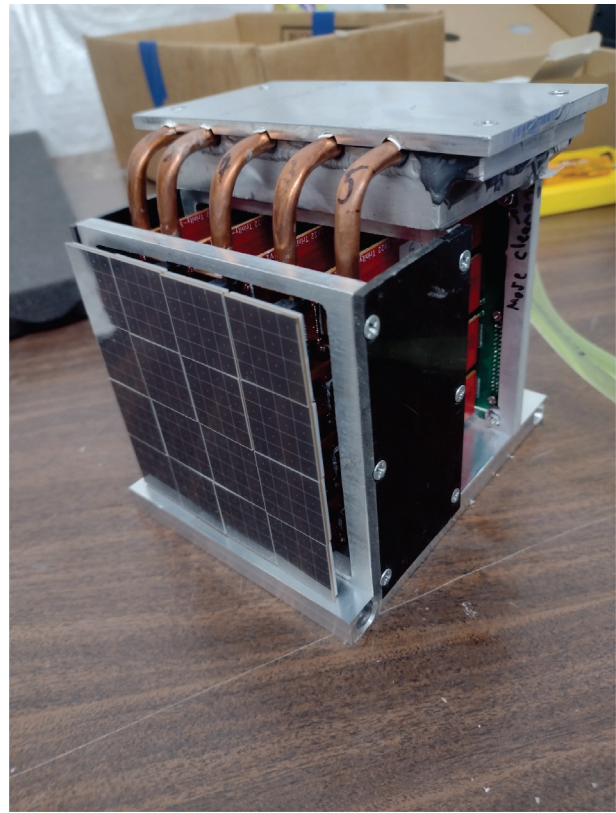
Fig. 7. The Demonstrator camera. The front of the camera consists of 16 SiPM matrices. The copper tubes are heatpipes, which are part of the camera cooling system.
