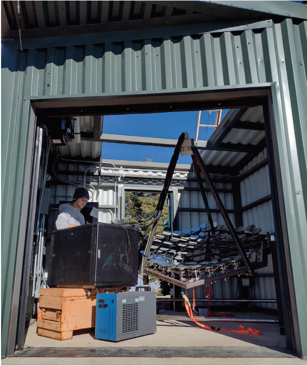
Fig. 27. The Demonstrator pointing at a \sim 30^\circ zenith angle to record air shower images from cosmic rays.
