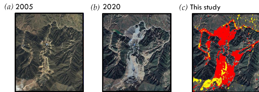
Figure 11. (a) Google Earth image for Mine site A in 2005; (b) Google Earth image for Mine site A in 2020 illustrating mine area expansion; (c) surface mine area expansion analysis result for Mine site A from this study, depicting surface mining extent in 2005 (visualized in yellow) and surface mining extent in 2020 (visualized in red).
