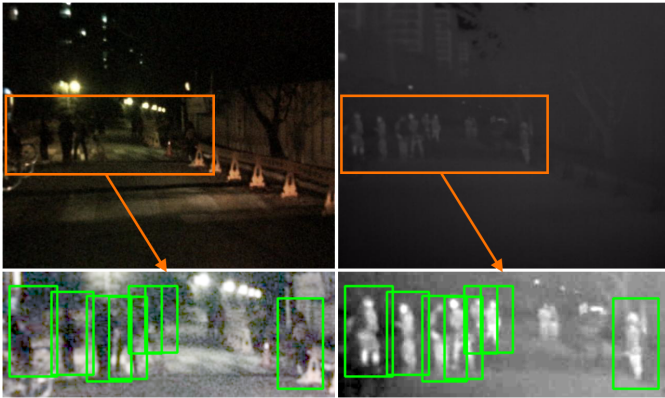
Fig. 5: KAIST Pedestrian RGB and thermal image pair with ground truth bounding boxes. The images containing the green boxes are over exposed for easier viewing.
