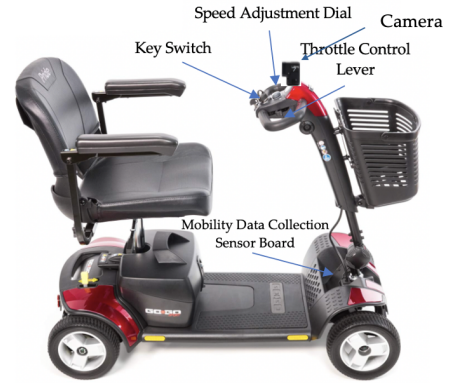
Fig. 2. Mobility Scooter with Camera and Motion Sensors Setup
