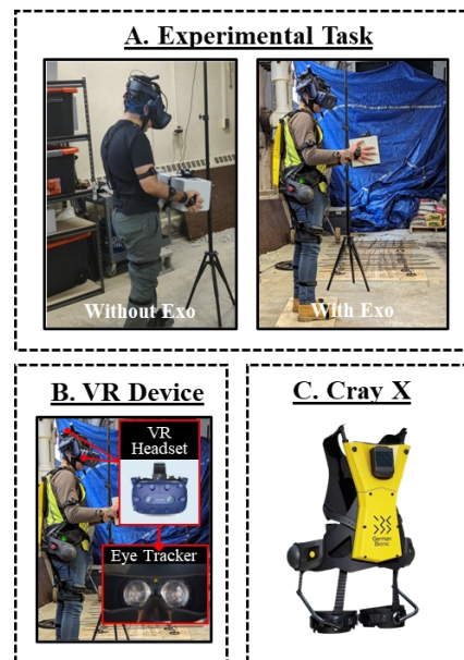
Figure 3. Vigilance Level Assessment Illustration (A) Experimental Task Setup (With and without active exoskeleton); (B) VR Device; and (C) Cray X exoskeleton
