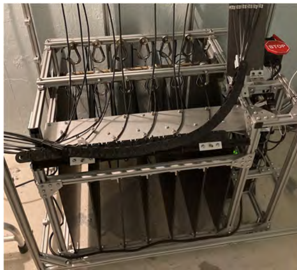
Figure 10. The KPF fiber agitator. Left: Front view showing the six fiber paths through the device. The science, sky and simultaneous cal fibers are agitated, and three backup copies of these fibers are also threaded through the agitator (but held away from the rotating bars). Right: A side view showing the rotating reel, which has two bars which tap the fiber loops. To minimize contact friction, the reel features PEEK tubing sections which independently roll as they contact each fiber cable.
