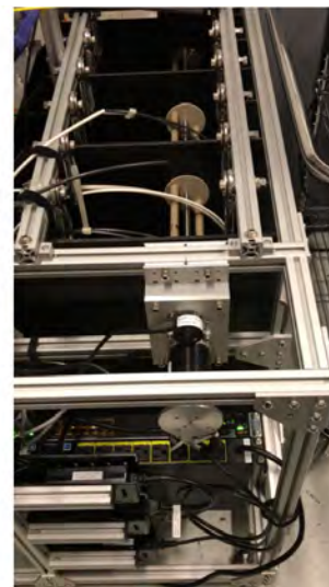
Figure 10. The KPF fiber agitator. Left: Front view showing the six fiber paths through the device. The science, sky and simultaneous cal fibers are agitated, and three backup copies of these fibers are also threaded through the agitator (but held away from the rotating bars). Right: A side view showing the rotating reel, which has two bars which tap the fiber loops. To minimize contact friction, the reel features PEEK tubing sections which independently roll as they contact each fiber cable.
