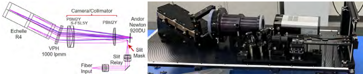
Figure 20. The optical design of the Calcium H & K spectrometer and the as-built instrument (with echelle grating cover in place). The larger camera lenses are 100-mm in diameter, and the R4 echelle grating measures 70 x 210 mm.
