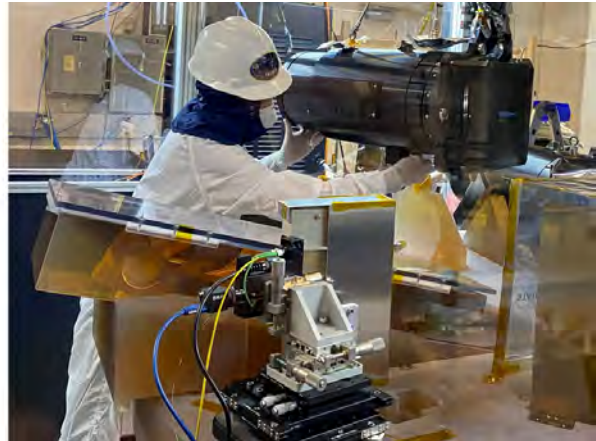
Figure 5. Left: Details of the KPF camera assembly. Right: The red camera assembly, supported by a crane during installation within the spectrometer. Also note in the foreground a Point Source Microscope (PSM) mounted on a multi-axis stage, which proved invaluable as a reformatter proxy during the early stages of spectrometer alignment.
