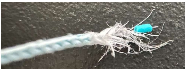
Figure 6: Mechanically broken sample of FOFL, the tight buffer (turquoise) is sheared in multiple places and the internal fiber optic core can be seen exposed.
