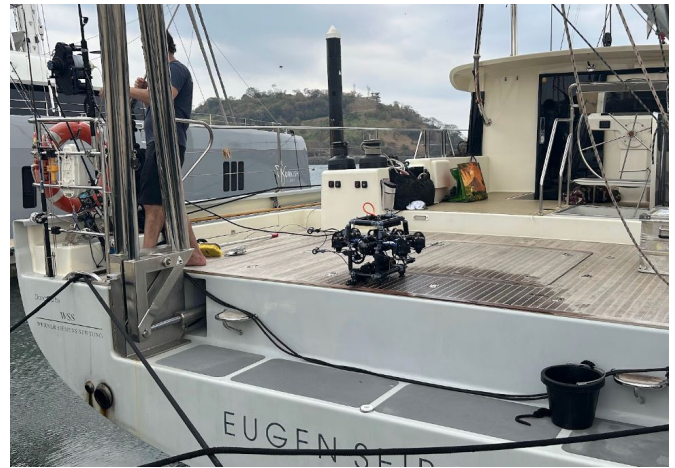
Fig. 10. ROV FiberFish sitting astern and the TMS with fiber-optic tether on the port stern the S/Y Eugen Seibold during pre-cruise set-up.
