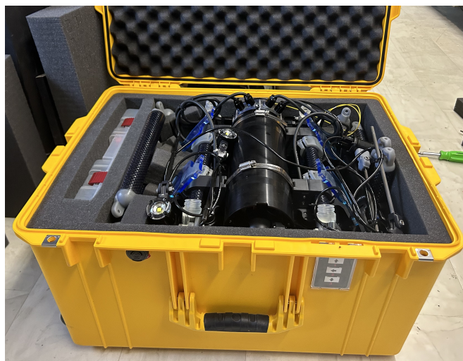
Fig. 4. ROV FiberFish packed into a Pelican 1637 Air case prior to transit. The ROV has been folded down, by design, to fit in this compact space and deploy readily and quickly once removed. An emergency tool kit was fit inside of the case alongside the vehicle.
