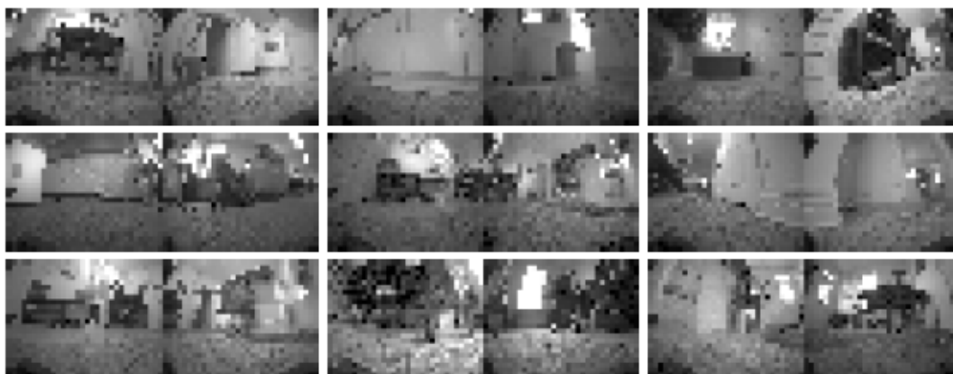
Figure 6.4: Example stereo video frames after processing. Stereo pairs are concatenated into a single image, converted to greyscale, then downsampled from the native resolution of 1232x3280 to 24x64 pixels.
