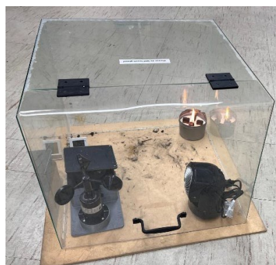
Figure 6: Photograph of the acrylic chamber with the sensors along with the small fire source, fan, and imaging. Suites implemented in actual fire detection will not be placed in the chamber; the system was used outdoors with the acrylic chamber was used to ensure the small fires were contained completely to maintain high safety standards.
