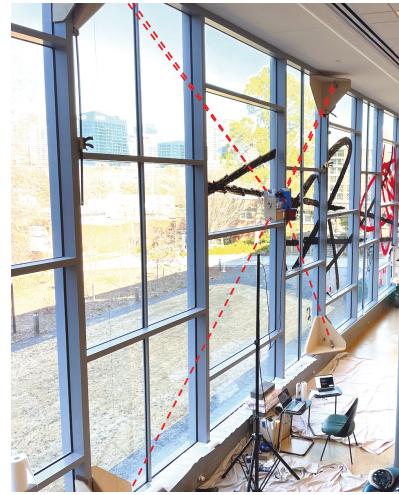
Fig. 2. Our 4-cable planar CDPR is 5.8m wide by 3.7m tall.
