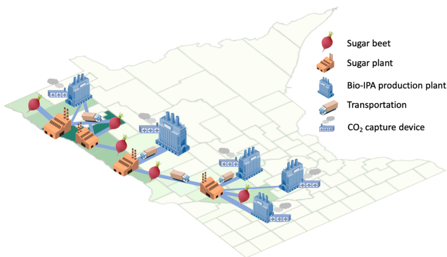
Fig. 1. The schematic representation of the three-tiered bio-IPA supply chain. The supply chain comprises sugar beet supply counties, sugar processing plants, and IPA production facilities. The optimization objectives include the costs and emissions associated with various sources: biomass, transportation, sugar production, IPA synthesis, and CO 2 capture processes.
