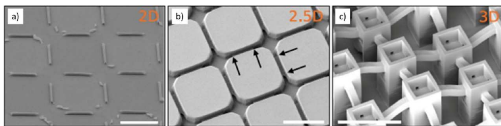
Figure 34. Scanning electron microscopy (SEM) images of devices utilizing spatial restriction in 2D, 2.5D, and 3D during cell culturing to control neuronal growth. (a) 2D pathways are defined by rolled-up GaAs/InGaAs microtubes. (b) Cavities and grooves with steps (arrows) are prepared by photolithography and reactive ion etching, defining 2.5D pathways for neuronal guiding. (c) Direct laser writing (DLW)-prepared scaffold structure with towerlike cavities connected by free-standing tunnels. The scale bars represent 50 \mu\text{m} . Original images are modified with permission from (a) Bausch et al. 804 Copyright 2013 AIP Publishing; (b) Fendler et al. 105 Copyright 2019 Wiley VCH Verlag; (c) Fendler et al. 112 Copyright 2020 Royal Society of Chemistry.
