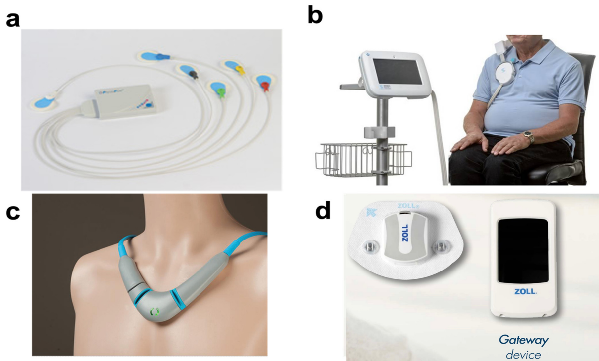
Figure 5. (a) PhysioFlow for measuring impedance cardiography [64]. (b) Remote Dielectric Sensing Vest for monitoring thoracic fluid index using electromagnetic beam [66]. (c) CoVa 2 for measuring thoracic fluid index and other hemodynamic parameters [67]. (d) Microcore for measuring thoracic fluid index and other cardiovascular parameters including ECG, HR, activity, and posture [68].
